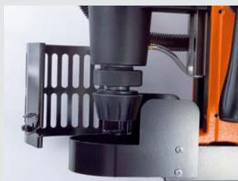
Increased operational safety through stable contact and swarf protection. (Optionally available as accessory)
