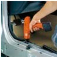
The positioning of the button for left-hand running makes quick switching to left-hand mode possible in the event of faulty screw drives. Single-hand operation is thereby made simple for left-handers too.
