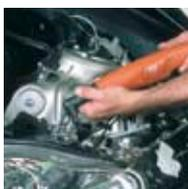
The LED illumination integrated into all screwdrivers lights up the screwdriving site perfectly. The view is perfect even in screwdriving spots where the view is usually difficult.
