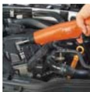
The offset construction allows for driving screws even in places which are difficult to reach. In addition the angled head can be adjusted by  $\pm 180$  degrees.
