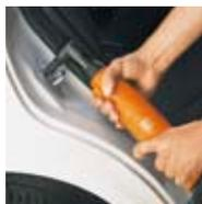
The outstanding ergonomics and weight distribution make single-handed operation possible. The standard soft start is easy on the hands and limbs of the operator and extends the service life of the motor and gears as well.
